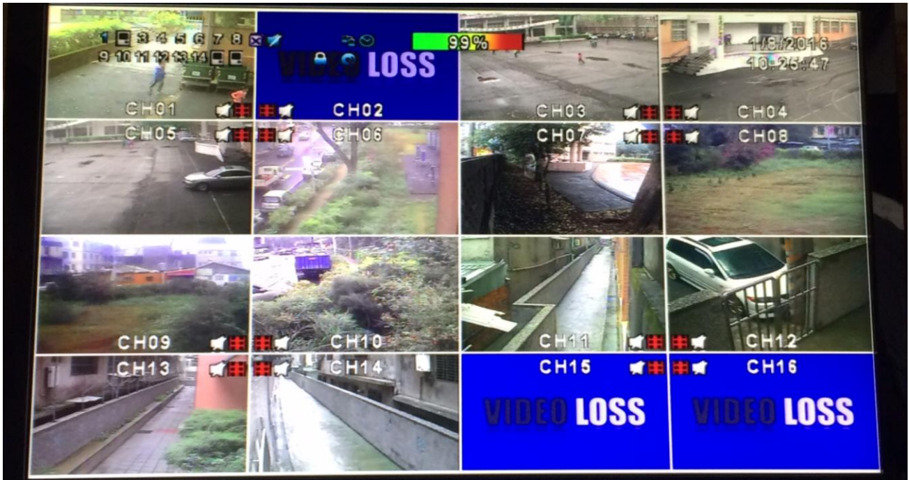
Figure 1. the original CCTV surveillance system. The signals of some channels became blurry and even disappear due to cable aging.
