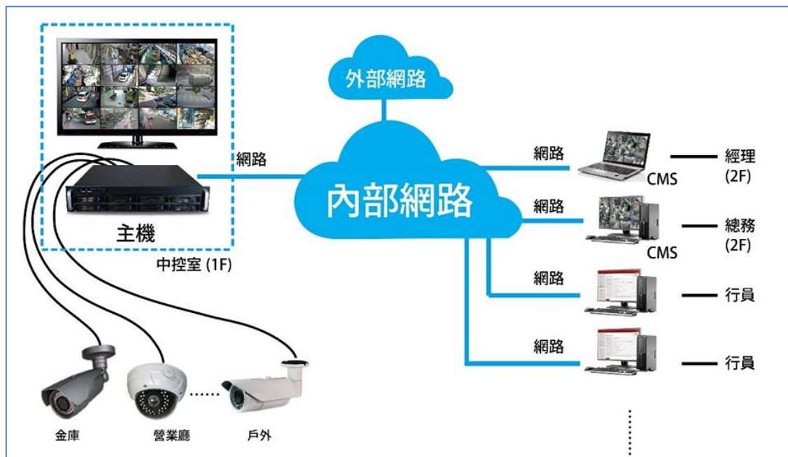
Figure 1. Block diagram of CCTV+CMS. The use of network may expose the surveillance system to the threat of hackers.
